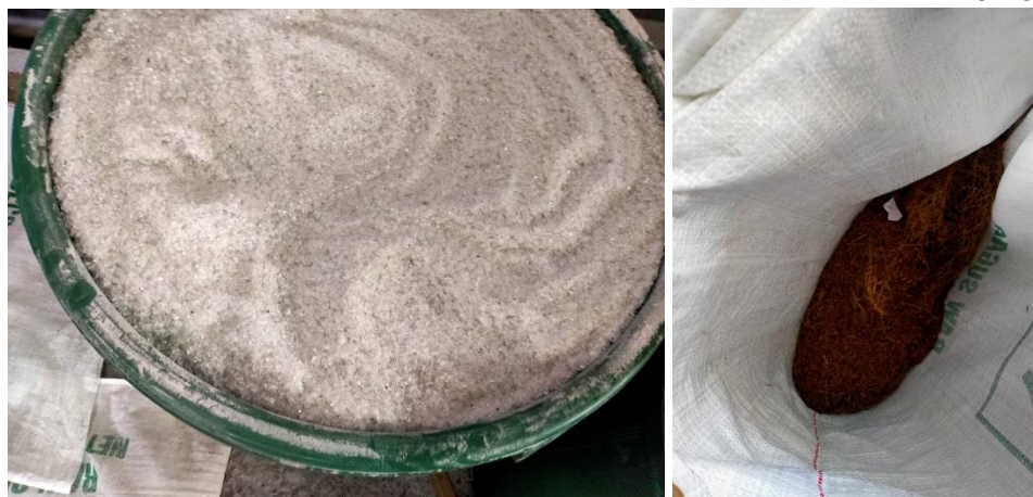
FIGURE 5. Sample raw materials processed by SWWABI – pulverized glass (left) and shredded coconut husk (right). / 14 June 2023
